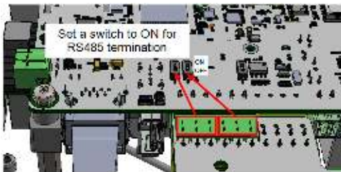
Figure 18: RS485 termination switch on inverter
