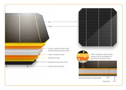
Panasonic HIT® KURO is the brand new all-black module which features a high module efficiency of 19.4%, an industry leading temperature coefficient of -0.258% /°C and a sleek design.
