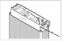
1. The small grommet is too small for an RJ45 plug to pass through. Without RJ45 plug at the end, feed the network cable through a small grommet and then through the top of the small cable entries.
