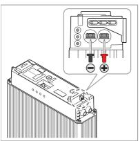
Measure the voltage at the terminal block using a voltmeter. If the voltage is lower than 38 V, do not use the battery pack. Contact LG Chem or your distributor.
