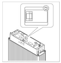
6. Press the circuit breaker's trip button. If the circuit breaker switch has not moved to the Trip position, do not use the battery pack. Contact LG Chem or your distributor.
