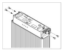
6. There are screw holes for mounting brackets on the top of the both sides of the battery pack. Drive the M5 screws through the mounting brackets into the holes and tighten them to a torque of 5 N·m.
