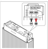
7. Measure the voltage at the terminal block using a voltmeter. If the voltage is higher than 0 V, do not use the battery pack. Contact LG Chem or your distributor.
