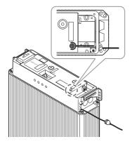
Grounding between the battery pack and the inverter is not mandatory but recommended.
