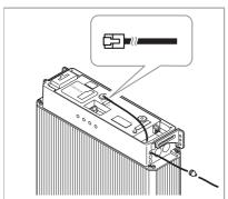
2. Attach an RJ45 plug to the network cable using a wire stripper and cable crimper. See Making network cable on page 18.
