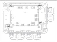
2. Loosen the screws at each corner of the metal plate that supports the circuit board. Be careful not to separate the circuit board from the metal plate.
