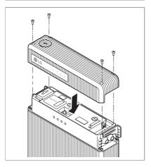
8. To secure the battery pack to the wall, replace the top cover and tighten the screws to a torque of  $2.75~\mathrm{N\cdot m}$ .
