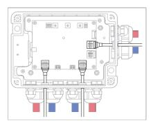
Connect each network cable to its corresponding network port. Use the port at the lower left for the first battery pack, the one at the lower right for the second battery pack, and the one at the upper for the inverter.
