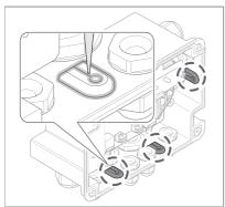
2. Apply silicone sealant or putty around the grommets and their slit.
