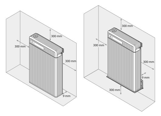
Make sure to leave a space of at least 9 mm between the battery pack and the wall. A clearance of at least 9 mm must be left around the battery pack for proper cooling.
