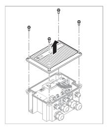
1. Remove the front cover of the RESU Plus. Loosen the screws at each corner of the cover and pull it up.
