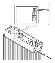
To supply power to the RESU Plus for its operation, connect the provided power cables from the battery pack to the RESU Plus.
