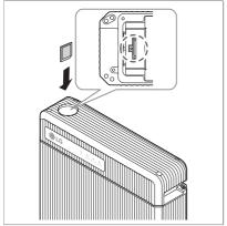
3. Insert the memory card into the memory card slot.
