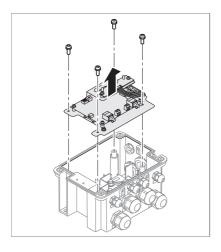
3. Pull up the circuit board to remove it.
