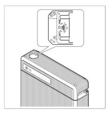
4. Press and hold the update button beside the memory card slot for more than 3 seconds.
