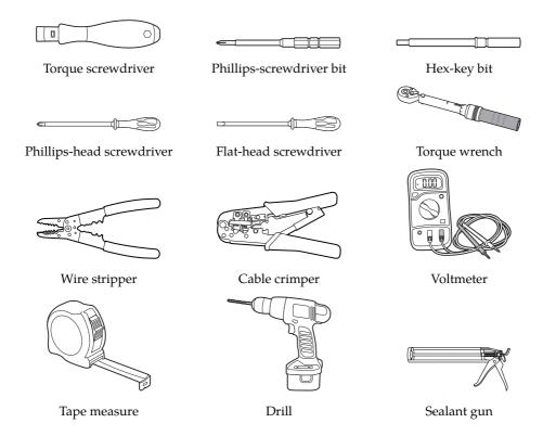
Use properly insulated tools to prevent accidental electric shock or short circuits. Use adjustable tools and measuring instruments that are certified for precision and accuracy.
