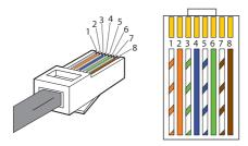
Use this method to make a network cable, which is to be connected between the battery pack and the inverter or the RESU Plus.
