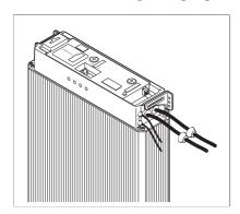
1. Feed a pair of charging cables through each of the large grommets and then through each of the large cable entries.
