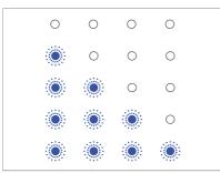
5. The LED indicators flash in cycles for 1 minute at most until the firmware update is complete. Only the **ON** indicator comes on when the firmware update is successful. If it fails, the **Fault** indicator comes on for two seconds. Check the memory card and try again. If it persistently fails, contact LG Chem or your distributor.
