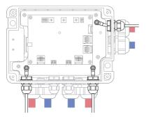
Grounding between the battery pack and the inverter is not mandatory but recommended.
