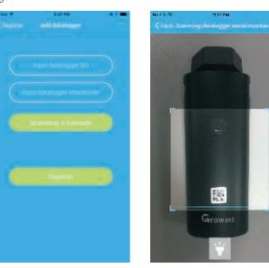
4. Fill out the required information, then click "Next", it will guide 5. Scan QR code or input the ShineWiFi-X barcode and checkcode, 6. Fill out the wifi network and password, then click "Configuration", after successful configuration, a note will pop up "Configured successfully", then it will move to the "my plant" page.
