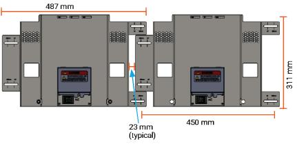
BWM-600MM-A allows 600 mm battery-to-battery spacing:
