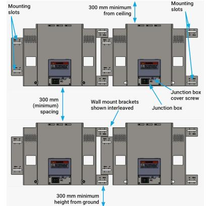
install the adjacent wall-mount brackets in an interleaved fashion, as needed. Be sure to align the mark on the adjacent wall-mount bracket to the centre of the wall stud. A small gap in between the adjacent wall-mount brackets is normal. You may install another row of wall-mount brackets above the one already installed. Maintain at least 300 mm (one foot) clearance between rows.
