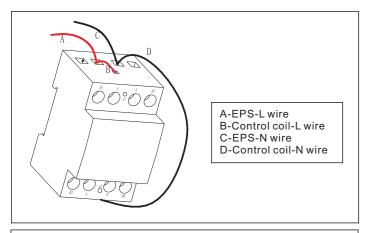
Use the screwdriver to unscrew the nut with position numbers A1, 3, A2 and 5 in the contactor, Then the red 12AWG wire ends are inserted into A1 and 3, both ends of the black 12AWG wire are inserted into A2 and 5, and tighten the corresponding nut with a screwdriver.
