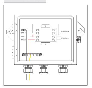
Use the screwdriver to unscrew the nut with position numbers R1 and R7 in the contactor, and then insert GRID-L wire and GRID-N wire into the port of contactor(R1&R7) through the cable nut and tighten them with screwdriver. Use a screwdriver to lock the ground wire on the E-wire copper bar.
