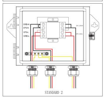
Use the screwdriver to unscrew the nut with position numbers 5 and 7 in the contactor, and then insert EPS-L wire and EPS-N wire into the port of contactor(5&7) through the cable nut and tighten them with screwdriver.
