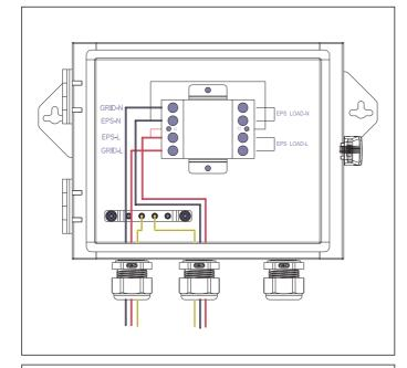
Use the screwdriver to unscrew the nut with position numbers 3 and 5 in the contactor, and then insert EPS-L wire and EPS-N wire into the port of contactor(3&5) through the cable nut and tighten them with screwdriver. Use a screwdriver to lock the ground wire on the E-wire copper bar.
