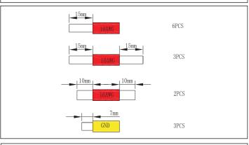
3. There are three types wire need to be machining, please check ref to 9.1 wired diagram. The follow three type wire are show as below:
