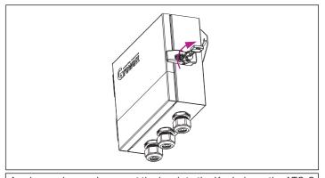
As shown above, please put the key into the Keyhole on the ATS-S right, clockwise rotation of 90°, the lower end of the first lock up gently move Open, remove the lock at the upper end of the buckle, then you can open the cover, Step of locking the cover opposite to the above.
