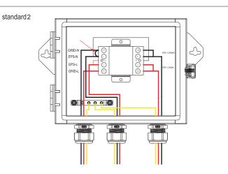
Standard 1 is for general using, and standard 2 is for like Australia where Neutral line can't be switched. When connect with ATS-S, please check which standard is suit for you.
