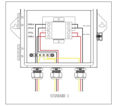
Use the screwdriver to unscrew the nut with position numbers 2, 4, 6 and 8 in the contactor, and the red 10AWG short wire ends were inserted into the contactor port 2 and 4, The Black 10AWG short wire ends were inserted into the contactor port 6 and 8, then insert EPS load-L wire and EPS load-N wire into the port of contactor(2&6) through the cable nut and tighten them with screwdriver. Use a screwdriver to lock the ground wire on the E-wire copper bar.
