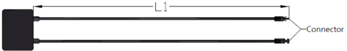
Fig. 13 (1) The full-cell module junction box
