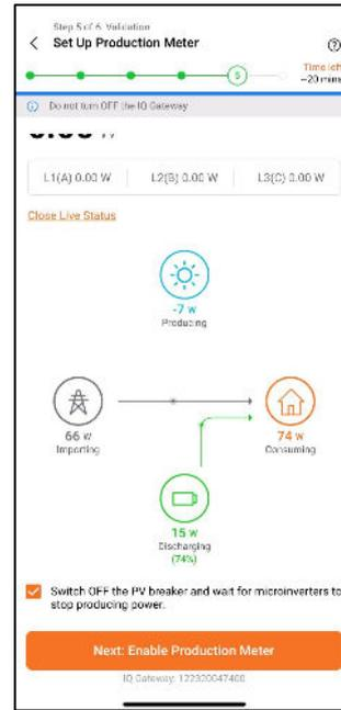
**Tap Next: Enable Production Meter after the production Meter after the production drops to Zero**
