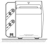
• This product includes a double isolation transformer, which meets safety requirements without array ground insulation resistance measurement and array residual current detection.
