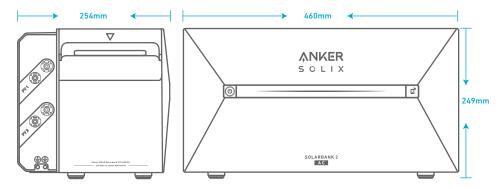
Figure: Anker SOLIX BP1600 Expansion Battery
