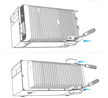
Note: When installing the bottom battery pack or only one Solarbank, please do not remove the bottom rubber plug to avoid water damage to the equipment.
