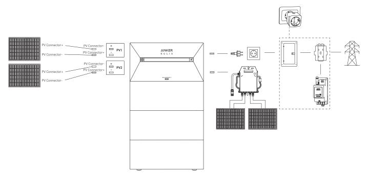
1. Connect Solarbank to the microinverter or a home outlet using the included AC Cable with Schuko plug (5m).
