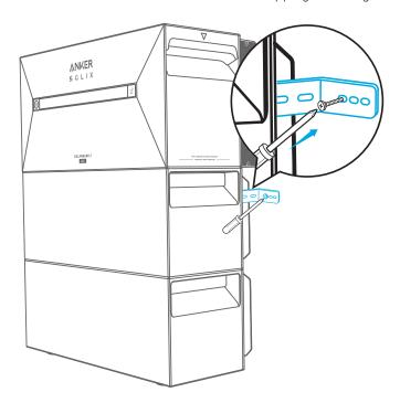
7. Use a Phillips screwdriver to fasten the M5×10 combination Phillips screws against the L-Shape Wall Mount Fitting; then secure the interlocking bracket to the expansion battery using the M5×10 combined Phillips screws to complete the installation.
