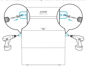
6. Use a hammer to tap the plastic sleeve of the  $M5\times60$  self-tapping expansion screw into the hole, and then use a Phillips screwdriver to fasten the  $M5\times60$  self-tapping screw against the L-Shape Wall Mount Fitting.
