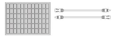
3. Connect each set of PV modules to each set of PV input ports in Solarbank using the included Anker SOLIX Solar Panel Extension Cable (3m).
