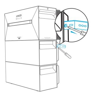
5. Mark the position of drilling holes on both sides and use a drill with a  $\phi 8$  drill bit and a depth of 60mm.
