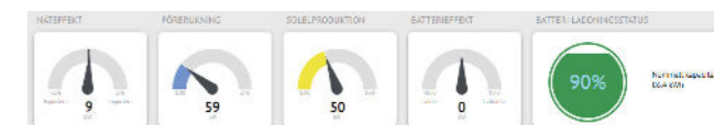
The dashboard displays real-time information on how much electricity you are buying or selling to the electrical grid, your energy consumption, solar electricity production and battery power in the property's EnergyHub system.
