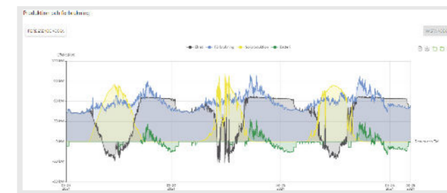
The power view allows you to see solar electricity production, electricity bought from and sold to the national grid and any battery, with second-precision going back one week.
