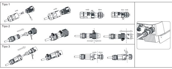
Suggest using 6mm² cables. Ensure the exposed core wire is totally inserted into the cable hole and connected securely.
