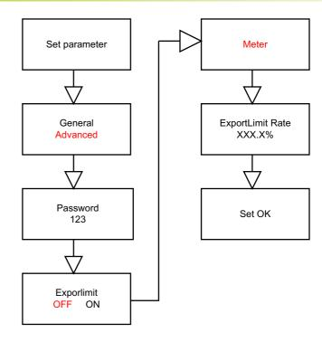
Under the permission given by your energy provider, the ratio of your system output power divided by the rated power of the inverter is called Export Limit Rate. For instance, if the energy provider only accepts 4kW from your 5KW system, then the Export Limit Rate of 5kW inverter is 80.0%.
